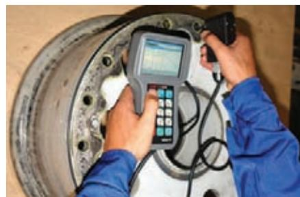
Circular scan permits an operator to locate the defect in the hole
