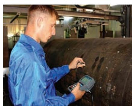
Carrying out of the main or confirmatory pipe body testing with the usage of VD3-71 flaw detector will enable to evaluate the pipe damage level and its further operability
