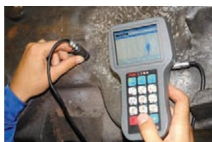
Usage of special-purpose PN-12-MDF 01 and PN-09-MDF 01 probes in protective cases together with ALARM units and digital signal processing will allow to eliminate the influence of interfering factors such as roughness, edge effect, ECP separation from the testing object surface etc.
